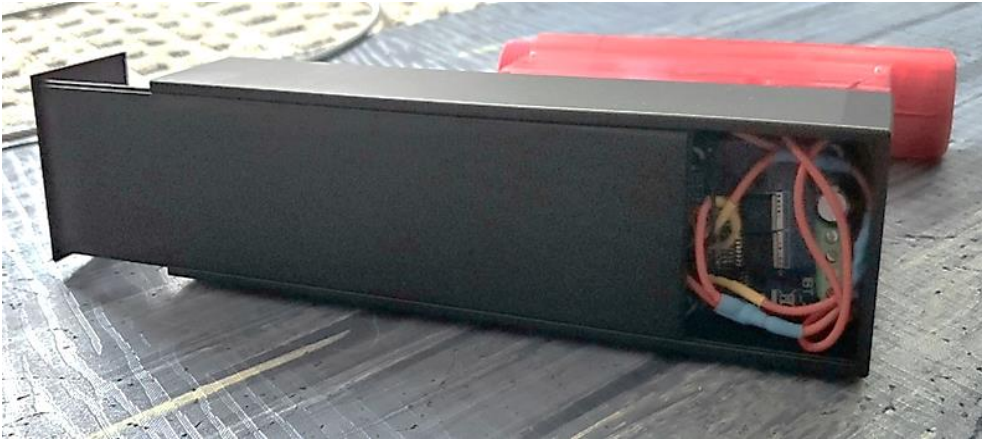
(Above) The 3D printed electrical box is shown attached to the final prototype with the sliding door cracked open. Inside the box includes the battery, pico-board, and motor controller
