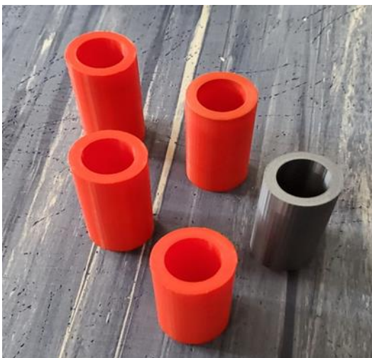
(Above) These versions of the launcher barrels all have slightly different inner diameters and thread styles. The correct version has .0625-11 inch thread and an inner diameter of 33.96 mm. The barrel correctly threads and fits to the final prototype with ease
