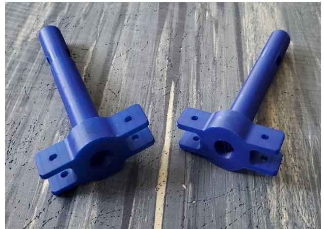
(Below) 3D printed "test shots" were made in different shaft diameters to accommodate the barrel of the firing system
