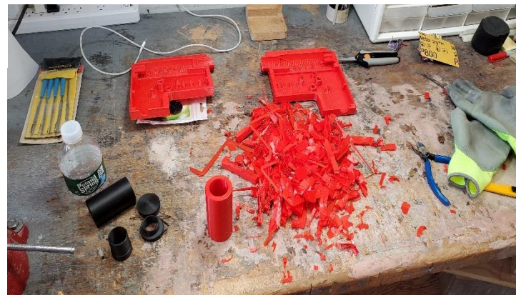
Removing PLA support (about 4 hours per set by hand)
