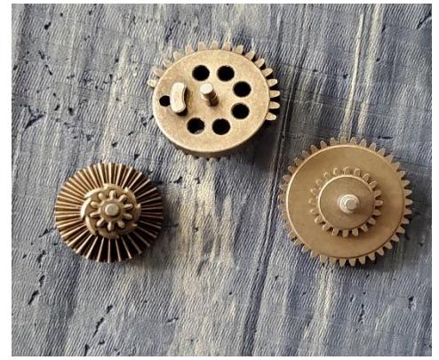
(Above) The first set of gears acquired by the team. These gears have a lower ratio (18:1) and are made from plain steel. The team later upgraded to Carbon-Steel gears with a higher ratio (26:1) to better accommodate the firing system
