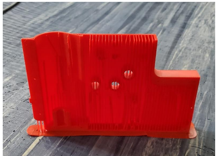
(Above) A failed 3D print attempt at the "V3" version of the housing. The printer had overheated and canceled the print at this exact point
