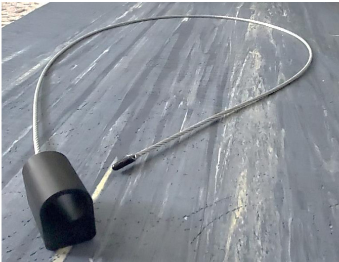
(Right) An industry grade zipline (5ft) is attached to a 3D printed cylinder that fits on the end of the metal grapple hook. The line is rated for 120 lbs. of payload
