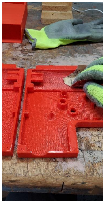
Sanding mechanism area (about 3 hours per set by hand)
