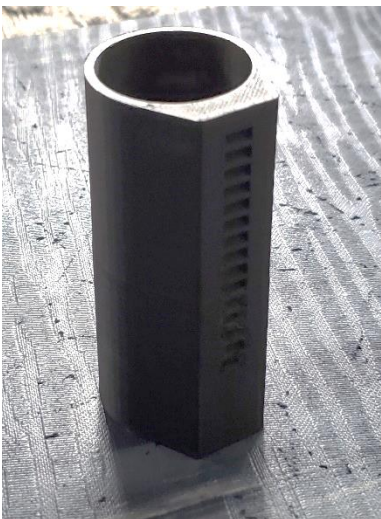
(Right) A Carbon 3D printed firing cylinder used for testing. The part had to be refined and re-printed to make better contact with the spur gear
